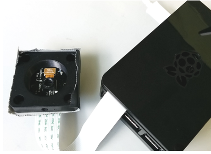
FIGURE 5.3: Image of the Raspberry Pi in its case with the connected camera module.
