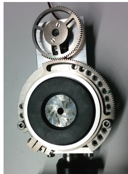
FIGURE 5.2: Image of the fully assembled aperture with mount and servo motor.
