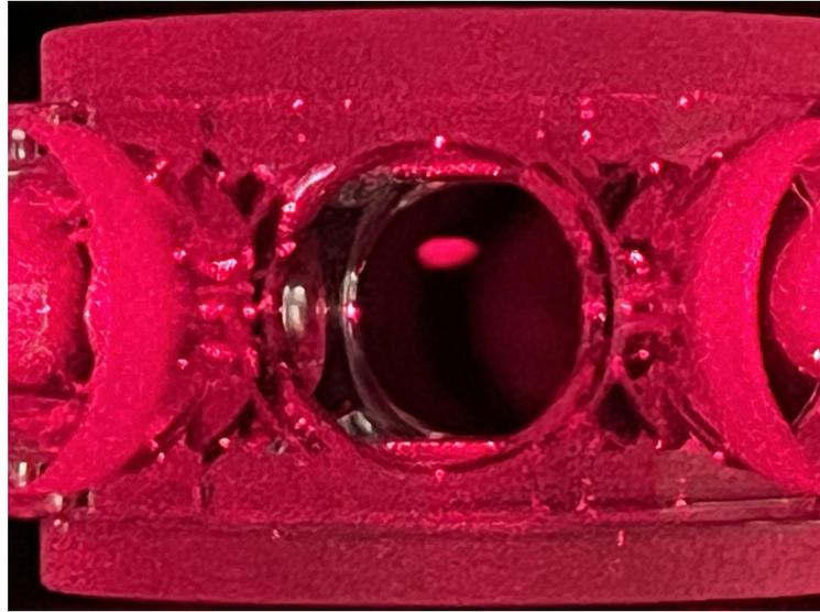
Figure 23: Picture of the 3D-MOT seen from a viewport of the glass cell.
